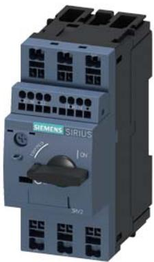
Circuit breaker size S00 for motor protection, CLASS 10 A-release 0.7...1 A N-release 13 A Spring-type terminal Standard switching capacity with transverse auxiliary switches 1 NO+1 NC
